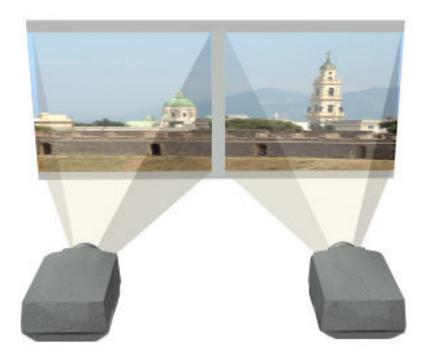
In this display, the projected images have a physical gap, so the Delta imagery must also have a gap otherwise things will not "disappear" properly in the gap.
