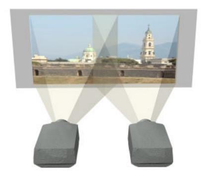
In this display, the projected images are physically overlapped (usually by 10%), then a blend is applied to the left & right edges to provide a seamless display.
